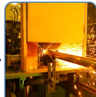
Automatic Pipe Cutting
